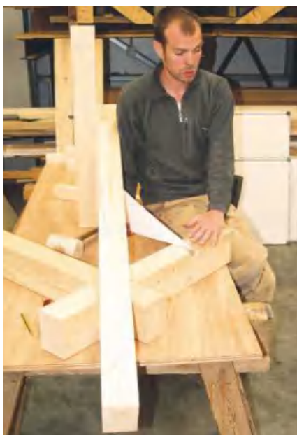
▲ Pic.1 Japanese carpentry works on centrelines. The first job, once all the timber has been squared up, was for Mathieu to snap a centreline using a sumi-sashi ink line. We used American tulipwood from Sydenhams timber yard, Maiden Bradley, because it is stable and clean. More about marking out can be found on Mathieu's blog: https://fabulalignarius.wordpress.com/2015/05/
